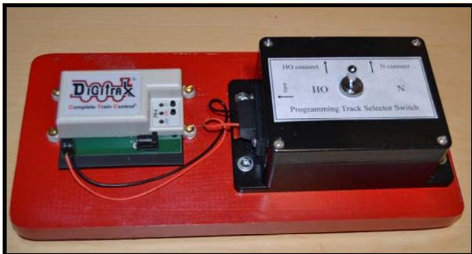
*PR4 Programming Interface and Programming Track Selector Switch*
