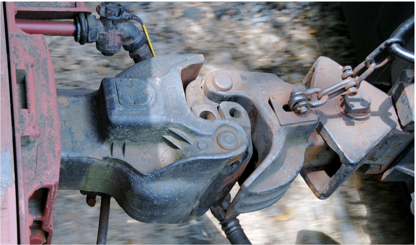
AAR Type E coupler (left) c. 1932, and a MCB Type 5 coupler (right) as required by 1893 Railroad Safety Appliance Act.
