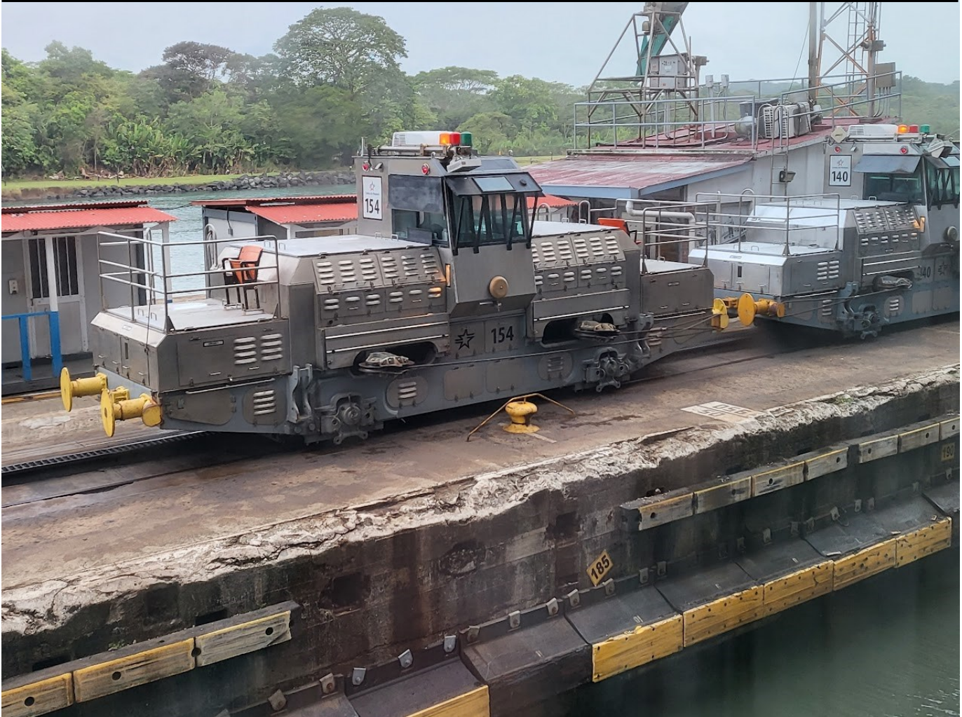
Panama canal “mule” used to guide ships through the original locks. The mules use a cog system between the 5 foot gauge rails to pull them up the 10% grade using electric power. Cruise ships usually have four mules attached but larger cargo ships have up to eight. All photos and facts on this page are provided courtesy of Jerry Enders.
