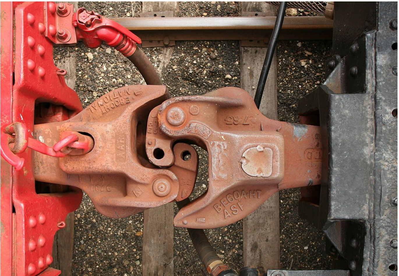
Mated Janney Type E couplers, as seen from above. Left is top-operated on locomotives. Right is bottom-operated on cars.
